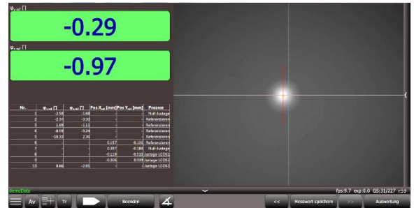
Fig.: Angular measurement with plane mirror
