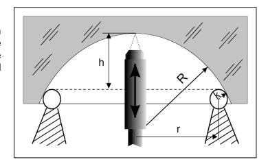
Measurement of the rise h is done by means of mechanical touching of the measurement and reference area with the aid of an incremental high-precision linear measuring system.
