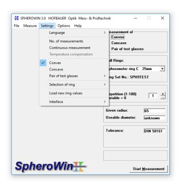
The user has the possibility of entering a desired number of repeated measurements and of tailoring the program settings to suit the measuring procedure: According to the choice of spherometer ring, ring type (ball ring, sharp edge ring), and according to the type of surface to be examined (convex / concave, pair of test glasses).
